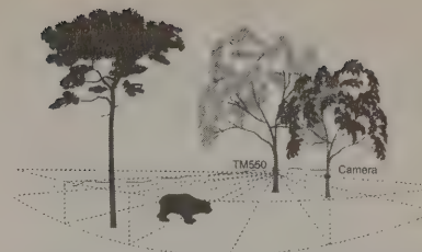
The TM550 must be mounted on a tree or post that does not move. The sensor is a heat-and-motion sensor and is dependent on being stationary to work properly. The camera can be located up to 25 feet away from the TM550.
